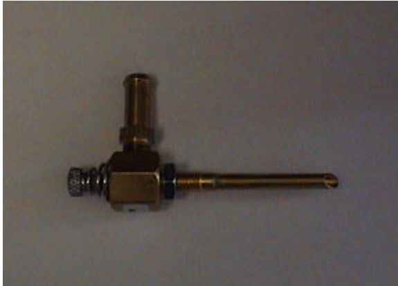
Figure 5: Jet with setscrew is on left
