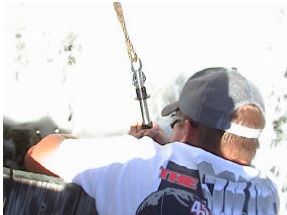
Figure 18: Static thrust test
