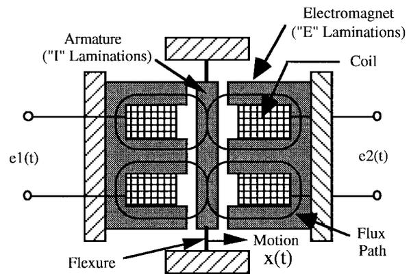
Fig. 1. Electromagnetic actuator based on attractive force.
