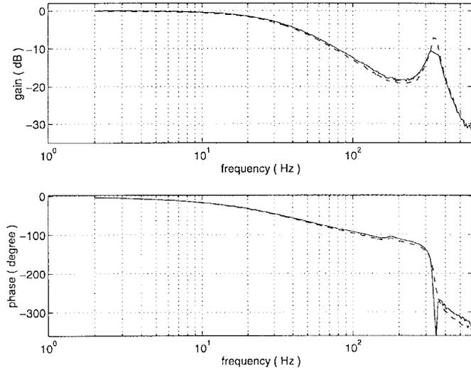
Fig. 6. Feedback linearization. Frequency response (measured response: solid line, least-squares linear fit: dashed line).
