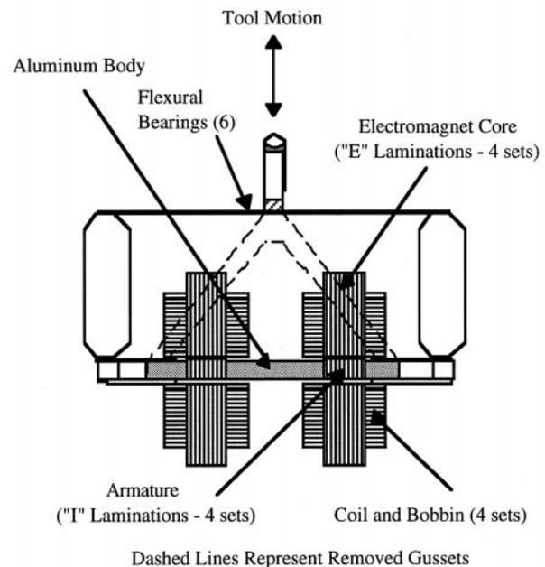
Fig. 2. Actuator schematic.
