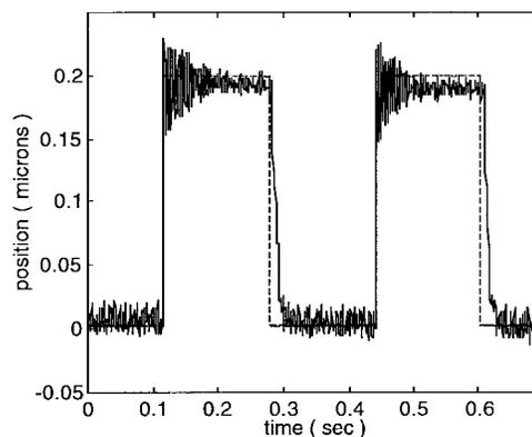
Fig. 4. Feedback linearization. Step response, 200 nm (reference command: dashed line, measured response: solid line).
