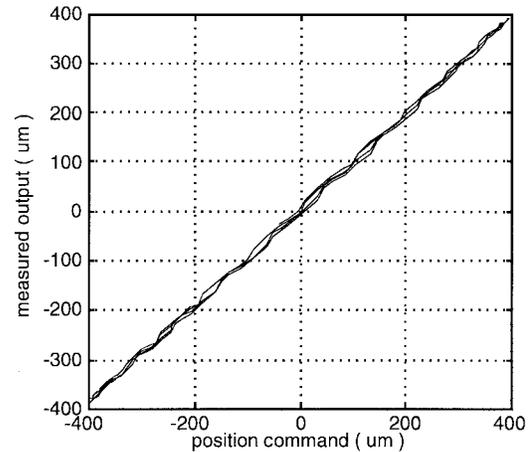
Fig. 10. Linearity of the closed-loop response, 800- $\mu\text{m}$  travel at 200 Hz.
