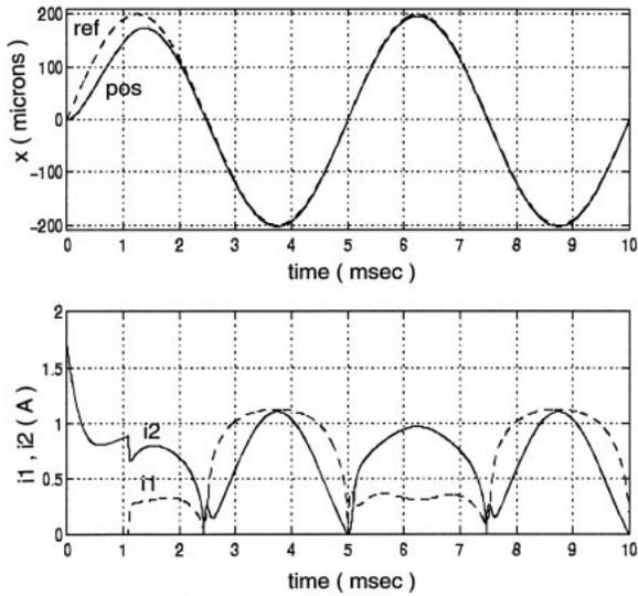
Fig. 7. Tracking performance, (16) 200- $\mu\text{m}$  sine wave at 200 Hz.
