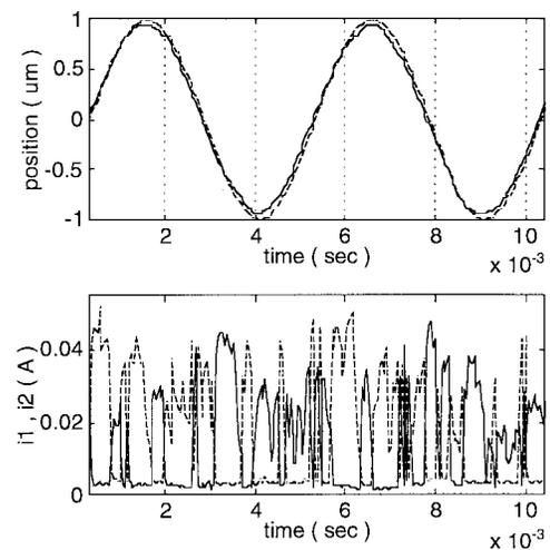
Fig. 11. Tracking performance: 2- $\mu\text{m}$  travel at 200 Hz.
