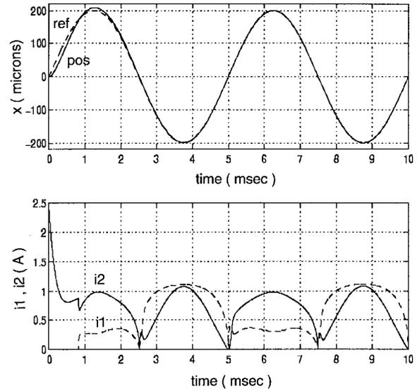
Fig. 8. Tracking performance, 200- $\mu\text{m}$  sine wave at 200 Hz. Sliding surface includes integral error term.
