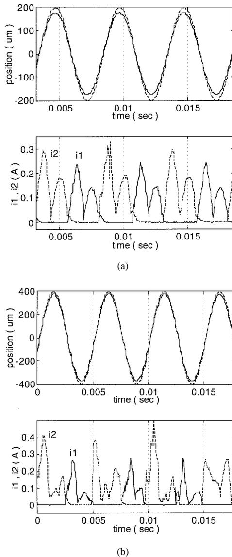
Fig. 9. (a) Tracking performance: 400- $\mu\text{m}$  travel at 200 Hz and (b) tracking performance: 800- $\mu\text{m}$  travel at 200 Hz.
