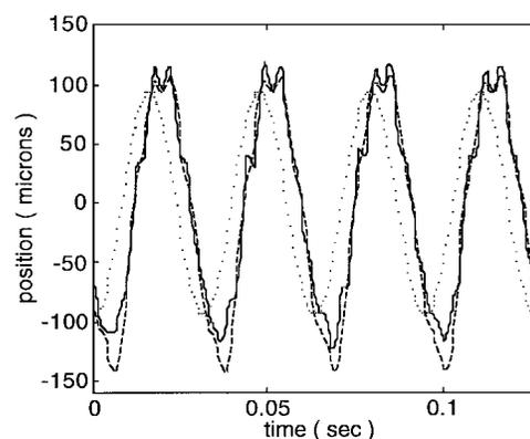
Fig. 5. Feedback linearization. Performance degradation (command: dotted line, measured output: dashed line, simulated output: solid line).
