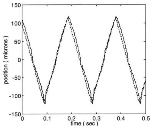
Fig. 3. Feedback linearization. Response to ramp command, 5 Hz (reference command: dashed line, measured response: solid line).
